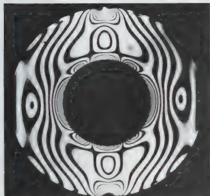
Photoelastic stress pattern of a ring in diametral compression
